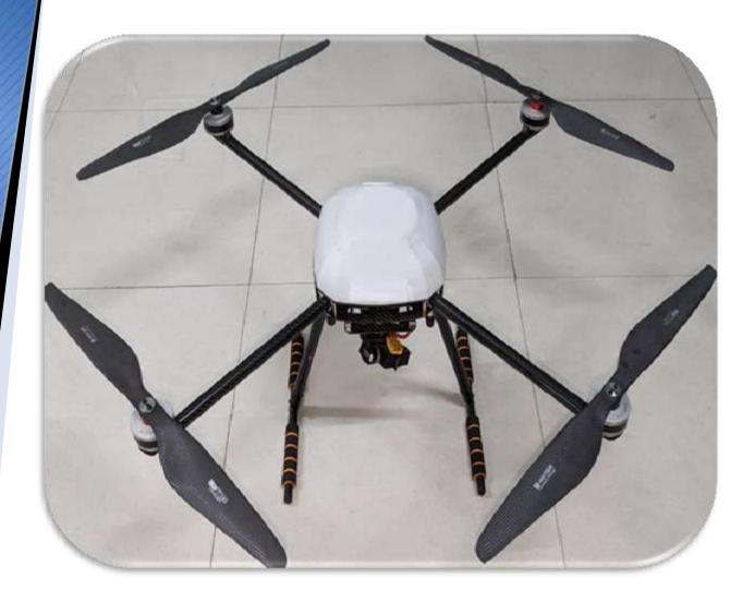
A Quadcopter, also called quadrocopter, or quadrotor is a type of helicopter that has four rotors. Although quadrotor helicopters and convertiplanes have long been flown experimentally, the configuration remained a curiosity until the arrival of the modern UAV or drone. The small size and low inertia of drones allows use of a particularly simple flight control system, which has greatly increased the practicality of the small quadrotor in this application. The Specifications are as follow.
